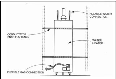
Flatten 1" at each end of the conduit and bend 45 degrees.
